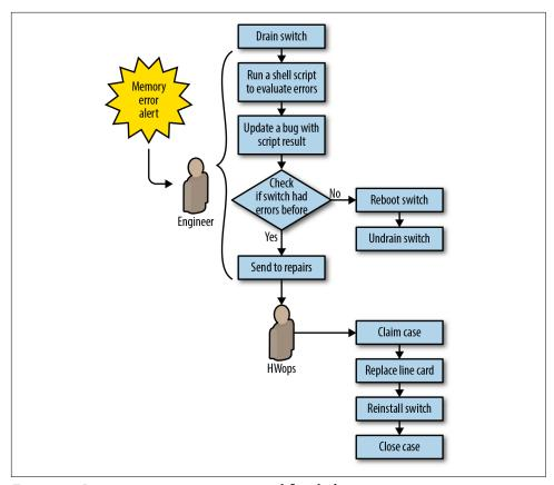
Figure 6-6. Jupiter memory error repair workflow before automation
