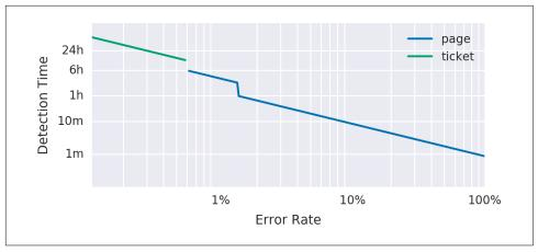
Figure 5-5. Error rate, detection time, and alert notification
