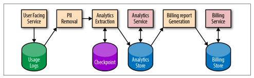
*Figure 13-2. Pipeline system diagram (PII = personally identifiable information)*
