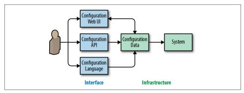
Figure 14-2. Configuration flow with a separate configuration interface and configuration data infrastructure. Note the web UI typically also displays the current configuration, making the relationship bidirectional.
