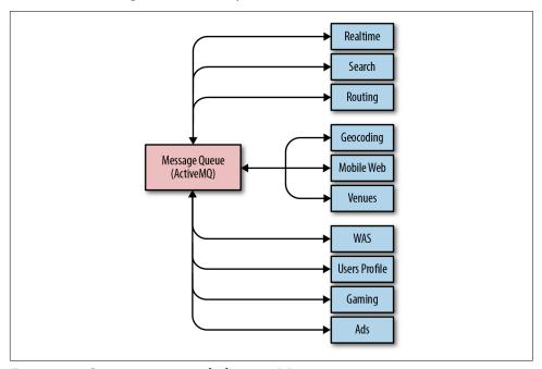
Figure 21-2. Communication paths between Waze components
