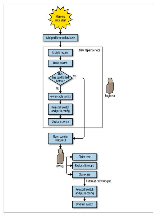
Figure 6-7. Jupiter memory error repair workflow with automation
