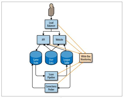
Figure 2-2. How our monitoring system collects SLI metrics
