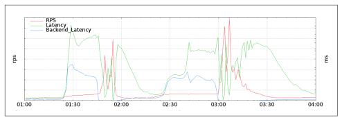
Figure 11-6. Traffic spikes caused by synchronous client retries
