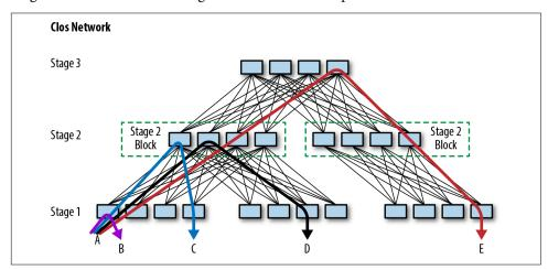
Figure 6-2. A small Clos network, which supports 480 machines attached below Stage 1
