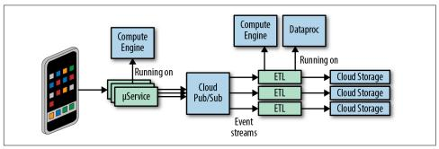
Figure 13-6. Event delivery system architecture
