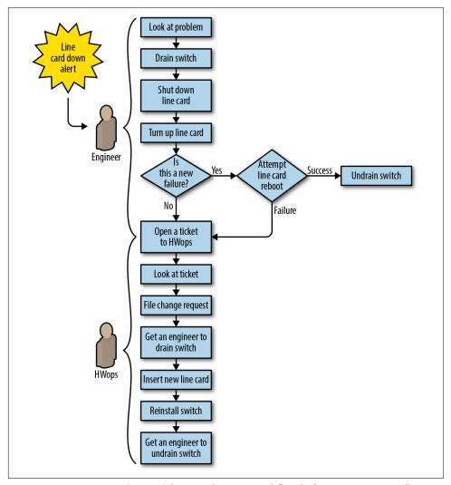
Figure 6-3. Datacenter (Saturn) line-card repair workflow before automation: all steps require manual work
